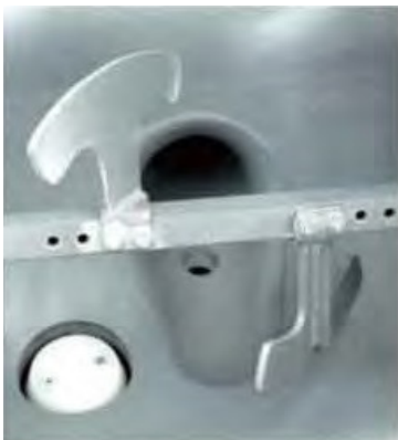
New design hopper with lower suction mouth to reduce remaining concrete level
