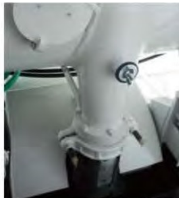
New design hopper with lower suction mouth to reduce remaining concrete level
